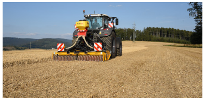
The CoverSeeder ensures a clean result. Crop residues are processed and remain on the surface.
