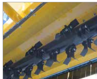
There is a lower suction effect thanks to the special Y-blades installed on the rotor and a variably adjustable working height of up to approx. 11 cm, meaning that reptiles and small organisms remain on the ground and do not come into contact with the Y-blades.
