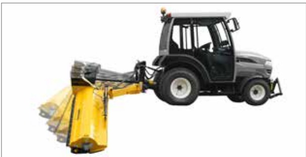
The patented mechanical collision protection device responds reliably and returns automatically to the working position.
