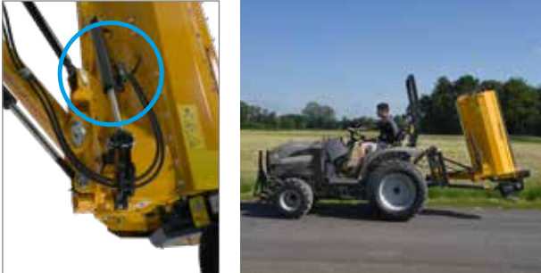
Secure transport lock for on-road driving or when transporting the tractor/equipment combination on a passenger car trailer.
