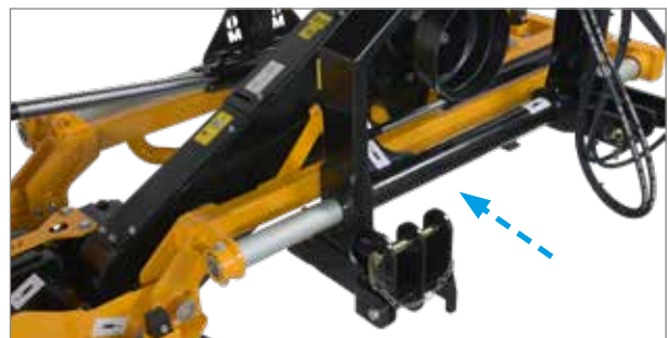
The mechanical collision protection device protects the mulcher effectively against collision damage if the worst comes to the worst.
