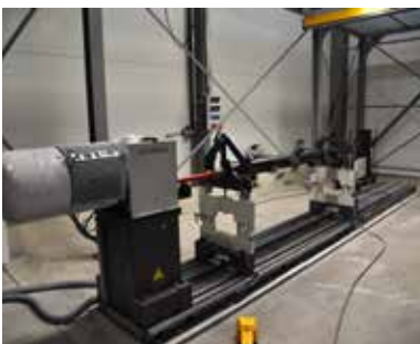
In-house balancing machine
