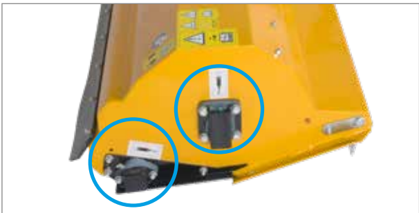
Easily accessible bearing points for quick maintenance.
