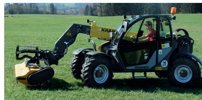
A low coupling point ensures good overall visibility due to the low linkage position.
