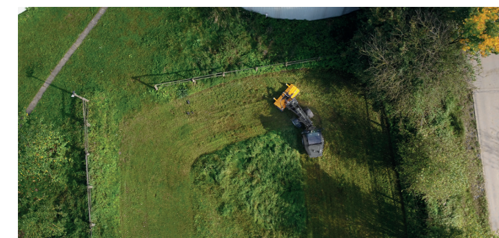
The mulcher follows the steering radius of the vehicle when cornering and the support roller does not scrape due to its low weight loading, thus protecting the ground.
