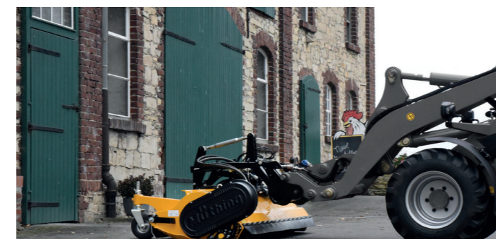
Custom-fit, vehicle-specific mounting parts make it possible to perform coupling quickly, without the use of tools and free of play in just a few seconds.
