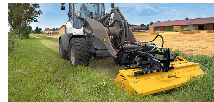
A unique feature is the patented virtual pulling point. Instead of being pushed, the mulcher is pulled with low rolling resistance and thus follows every ground contour perfectly.
