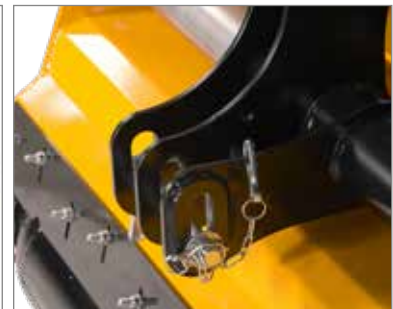
Elongated holes on the upper and lower link mounting points ensure excellent ground following in combination with the swivelling support roller.
