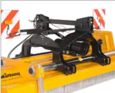
Sturdy front/rear headstock with hydraulic side shift (56 cm adjustment range) and Cat. 2+3 mounting points.
