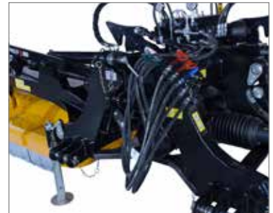
Tidy: The on-board hydraulics with the hydro-pneumatic MU-SOFA® weight transfer system.
