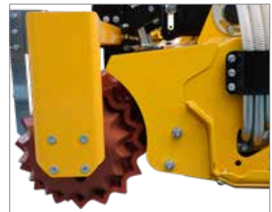
Dust protection - Extension at flail mower housing reduces dust generation and soiling.
