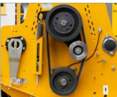
Trouble-free and low-maintenance operation due to the efficient design of the automatic belt tensoning system.
