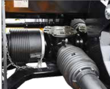
The clever design allows for a high-performance twin gear box and split power transmission to each side.
