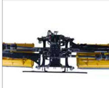
The clever offset design allows for a high-performance twin gear box and split power transmission to each side.
