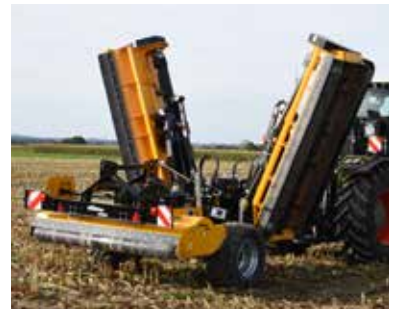
Folds in and out quickly to achieve a transport width of less than 3 m.
