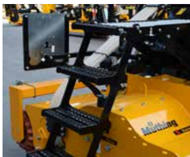
Easy filling of seed tank thanks to a folding step.
