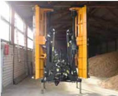
A clever design allows the MU-PRO/F Vario flail mower to be folded up for space-saving storage.
