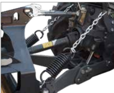
The front shock-absorbing spring assembly provides optimised ground adaptation and leads to better traction and steering characteristics of the tractor by loading the front axle (optional).
