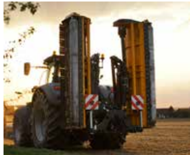
Clever folding: Minimal equipment height due to the parallelogram-type suspension of the two flail mower housings.
