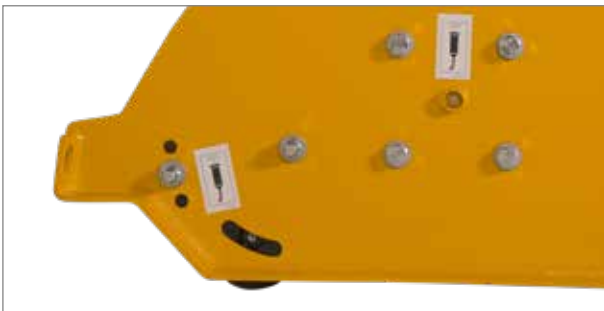
Adjustable support roller for depth control.
